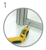
Affix first curved profile flush with bottom of both 8-way posts ensuring the cut out in both triangular stealth plates face inwards (as shown).
