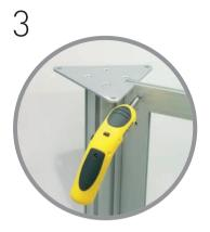
Attach second curved profile to both posts and both verticals ensuring the top of the profile is flush with the top of the triangular stealth plates. Tighten clamp screws to secure in place.
