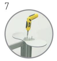
Align base plate to 8-way post in position shown. Insert 4 off fixing screws and fasten. Repeat for second base plate.
