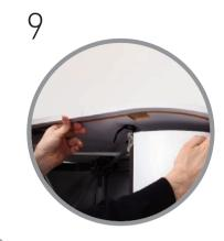
Align slots and channel in the underside of table top with hubs and graphic, and carefully lower into position.
